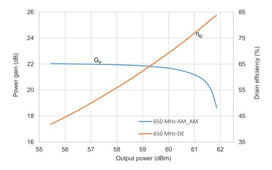
Fig 3. Power gain, Drain efficiency vs. CW output power
