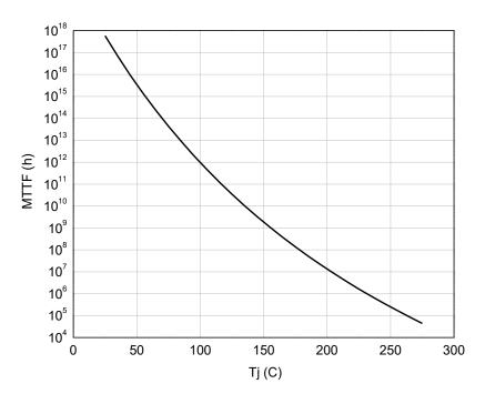
Fig 3. Median lifetime vs. channel temperature
